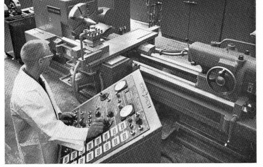
TAPE-CONTROLLED LATHE, recently installed in the Development Shops, is operated by John Malpas (4251-2) using the manual over-ride controls. The new machine has superior production capabilities and unique tooling capabilities.
